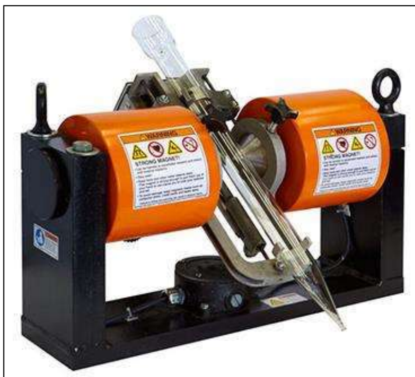
Figure 11-1: A Davis Tube Magnetic Separator
