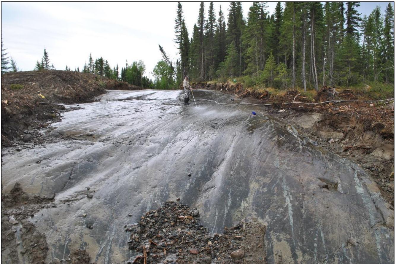
Figure 9-1: Washing of a stripped area of the South Zone deposit to expose the glaciated bedrock below
