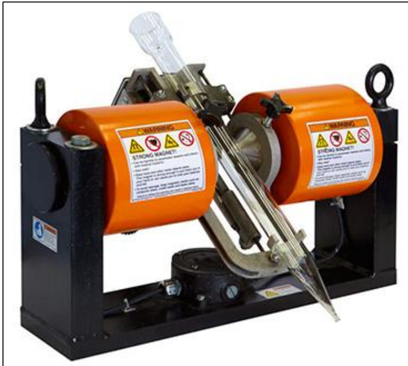
Figure 11-1: A Davis Tube magnetic separator
